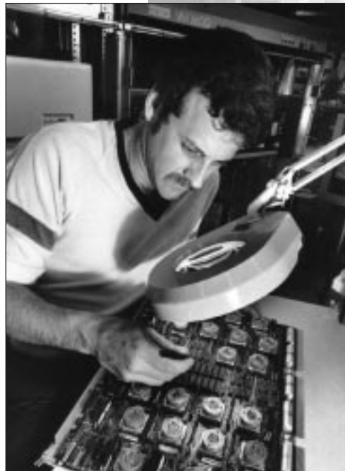
Field service engineer repairing customer CPU board.
