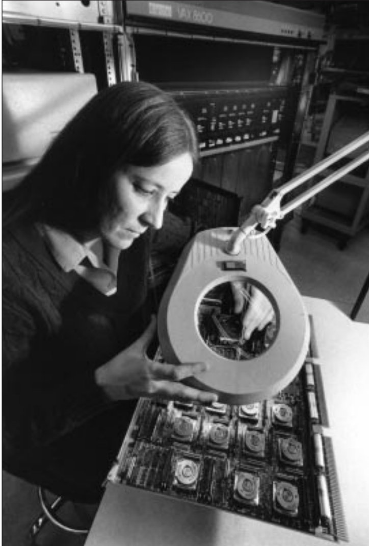
VAX quality control inspection of VAX 8600 CPU board.
